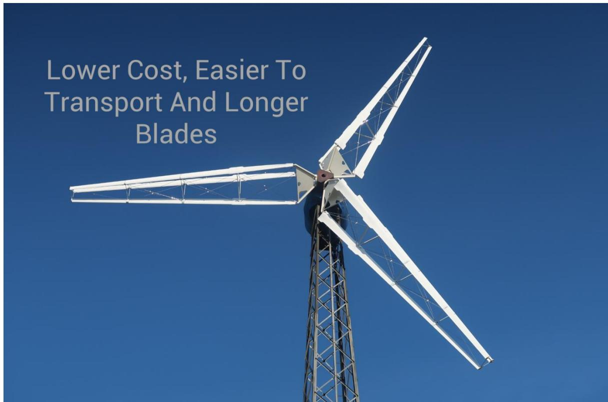
22m Triblade rotor on a wind turbine.
