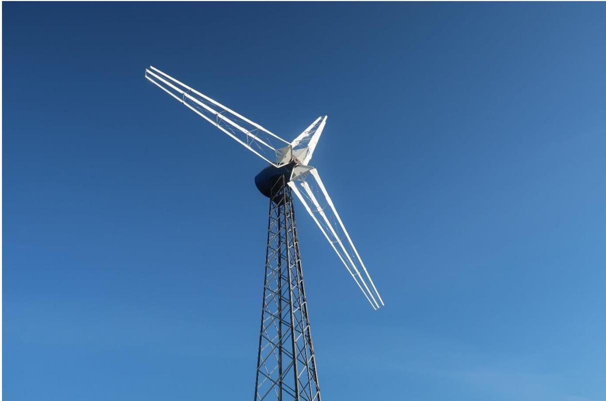
A complete 22m Triblade rotor installed on a wind turbine at test center in Denmark.
